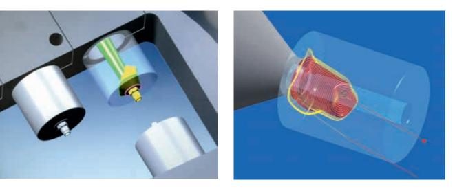
In the case of prefabricated abutments, the implant interface and screw channel have already been pre-milled, therefore, the lab or milling center only needs to finish the emergence, shoulder, and abutment body. This translates to faster manufacturing times, as the most intricate process has been completed. Additionally, *hyper*DENT<sup>®</sup> allows for prefabricated abutments to be milled using either multipart or single fixtures, providing even more flexibility and freedom of choice.
