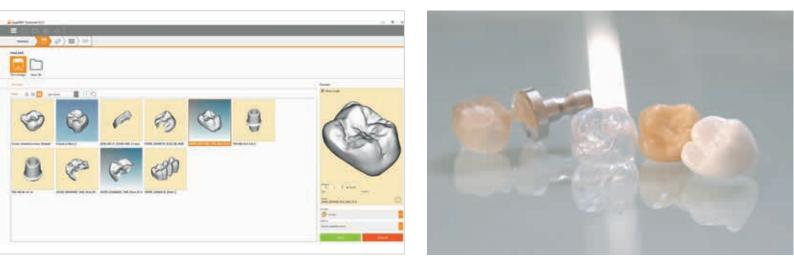
The ideal blank is recognized already during the automatic loading process and suggested to the user. The positioning of the blank and setting of the connector are also automated. For machines with multiple slots, multiple blanks can be loaded and calculated within a project, saving the user valuable time. Predefined milling strategies ensure high process stability and efficiency.
